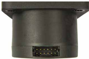
Fig. 1 Hirose DF11-12DP- 2DS9(24) header
